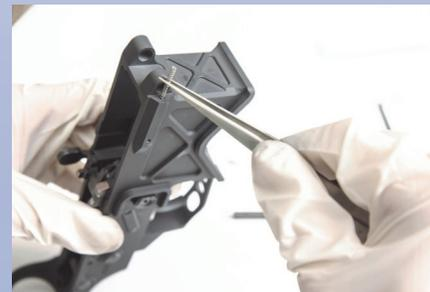
**6. Install the buffer retainer and extensions.** First, install the retainer and retainer spring inside the slot on the receiver, then hold it. Second, drive the extension just above the retainer to catch it. Third, install the buffer spring and buffer assembly inside.
